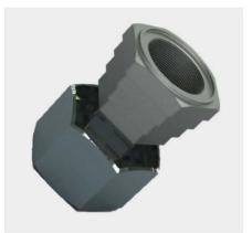
The two-part design consists of interlocking inner and outer sleeves with tapered threads that integrate advanced anti-galling properties. Compatible with standard bolt threads, the HYTORC Gall-Free Nut can be finished in a variety of coatings and materials to suit your specific applications.
