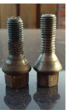
The HYTORC Gall-Free Nut coated thread design eliminates the microscopic material corrosion that occurs when fasteners are subjected to high temperatures and increased friction over extended time periods. This technology counters the galling effect of plastic deformation and micro-scale material transfer of thread surfaces.
