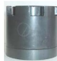
This requires the use of square adapters which fit the cogs of the inner sleeve. This ensures that the sleeves do not become misaligned with each other.
