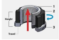
The HYTORC Nut is composed of an inner sleeve (1), outer sleeve (2), and washer (3). As the outer sleeve turns (blue arrow), the inner sleeve moves upwards (red arrow). The washer spline rotationally couples the inner sleeve with the washer preventing the inner sleeve from turning while providing a solid reaction point for turning the outer sleeve.
